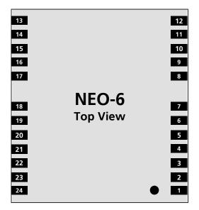
Figure 2 Pin Assignment
