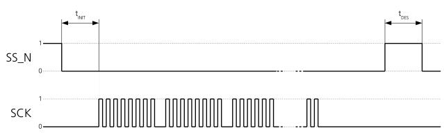
Figure 3: SPI timing diagram
