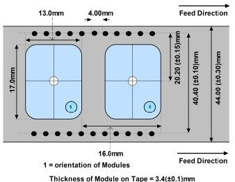
Figure 7: Dimensions and orientation for NEO-6 modules on tape
